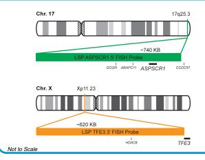
LSP ASPSCR1 5' FISH Probe covers the entire ASPSCR1 gene and some genomic sequences adjacent to the 5' (start) and 3' (end) of the gene. LSP TFE3 3' FISH Probe covers the 3' (end) part and sequences downstream of the TFE3 gene. The probe set is optimized to reveal translocations between the two genes.
